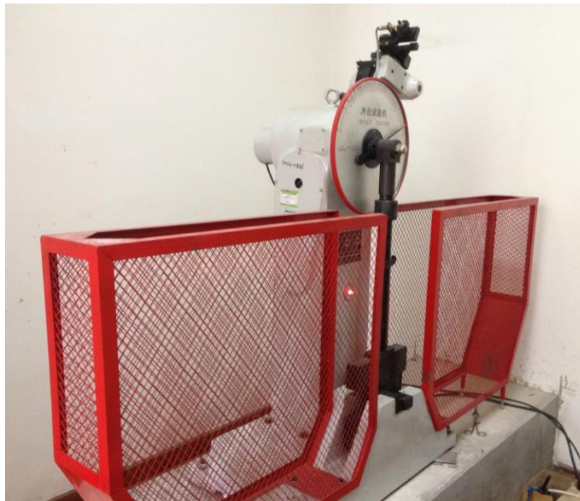
Figure 21. Standard pendulum impact tester used in this work.
